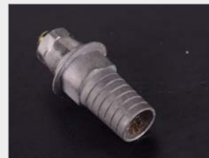
14 Alpha-Bio Tec Ti-base abutment sandblasted with 50 µm aluminium oxide (pre adhesive cementation).
