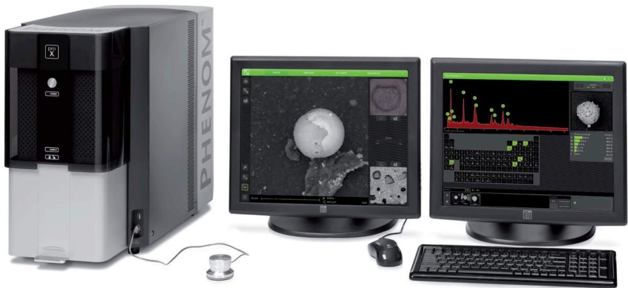
Workstation with Phenom proX Scanning Electron Microscope
