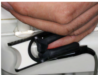
7 Fig. 3a: Electric sensor to monitor arterial blood pressure, pulse and oxygen saturation.
