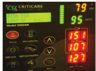
9 Fig. 3c: Oxymeters to monitor arterial blood pressure, pulse and oxygen saturation.
